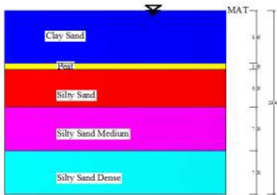
Gambar 3.1 Lapisan Tanah Eksisting (Maricar dkk, 2014)
